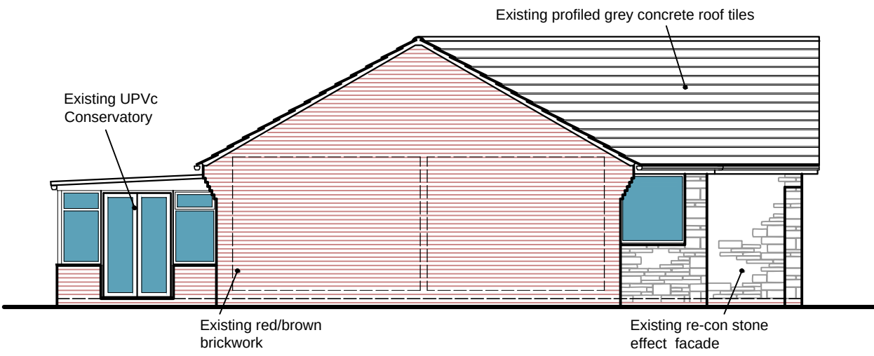
Existing East Elevation
