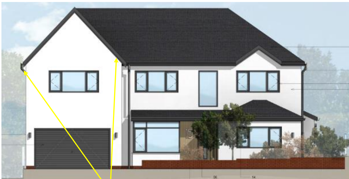
Proposed front elevation, indicative sites of replacement roosts, see below Bat access sited such that they are not directly above doors or windows.
