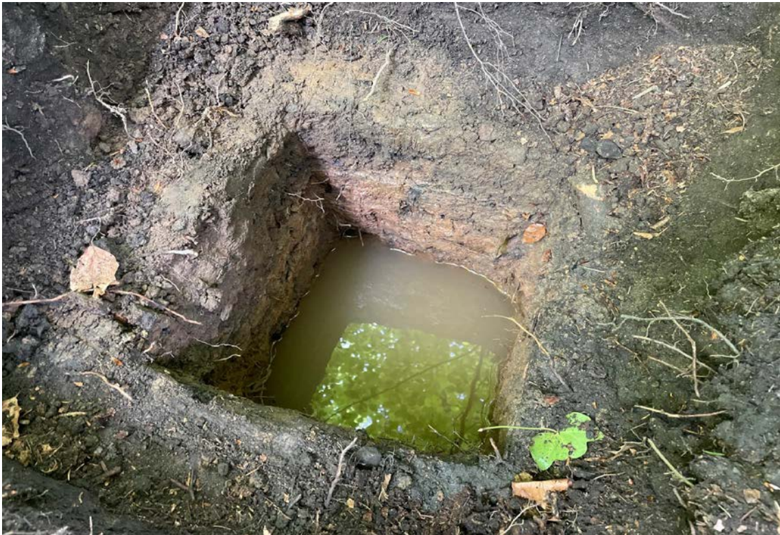
Photograph 4 – Each soakaway test was terminated when 75% effective empty depth was reached.
