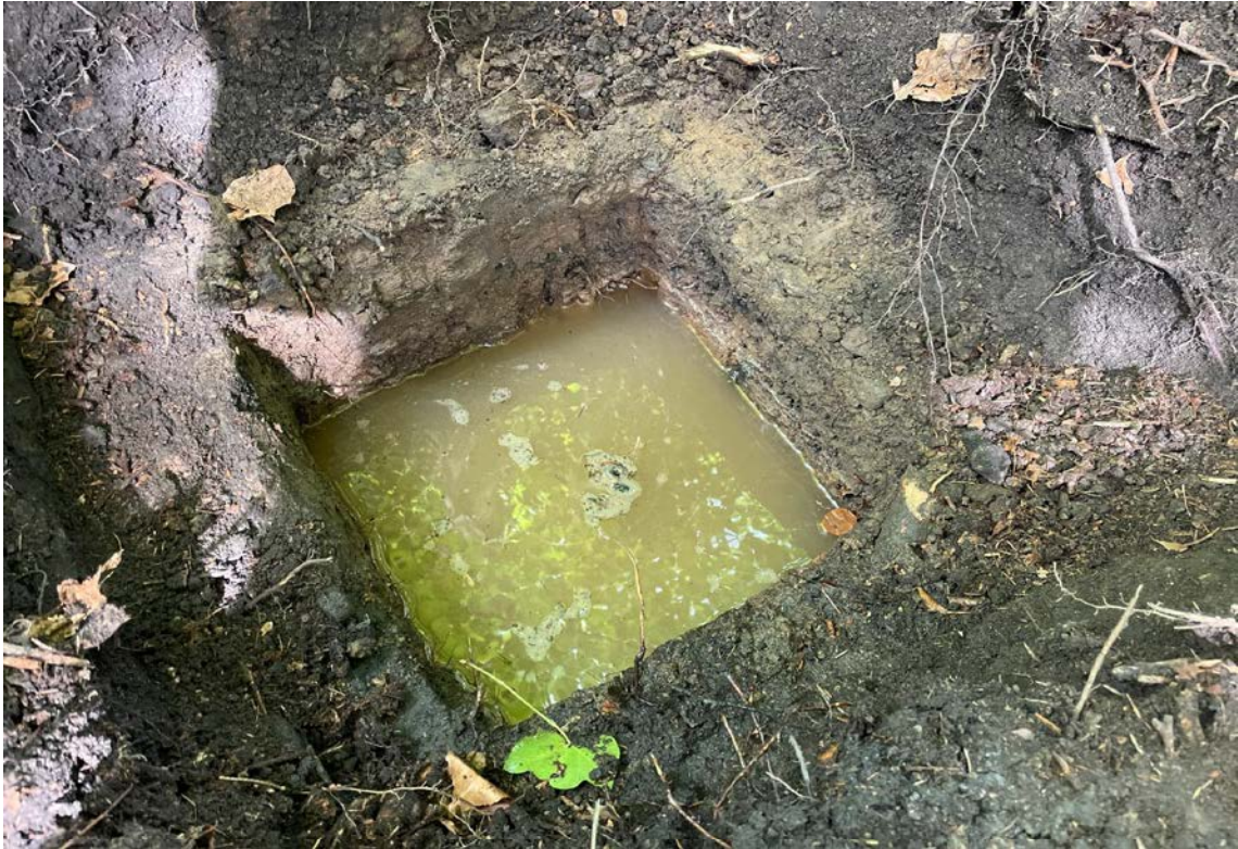
Photograph 3 – The water level was filled up to around 0.1m below topsoil level for each test, targeting the glacial strata.
