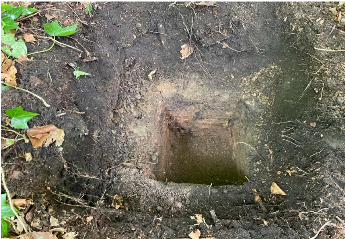
Photograph 2 – A soakaway test pit with an area of 0.3m 2 was excavated into the glacial deposits, with a depth of 0.4m below topsoil level (0.65m below ground level).
