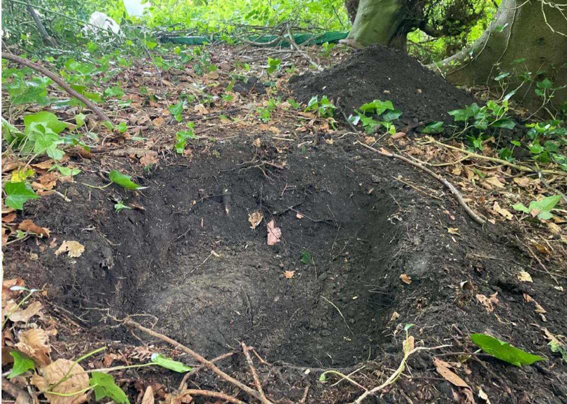
Photograph 1 – The upper boundary of the glacial clay can be seen underlying the topsoil strata. Depth measurements were taken from a fixed datum at the bottom of the topsoil.
