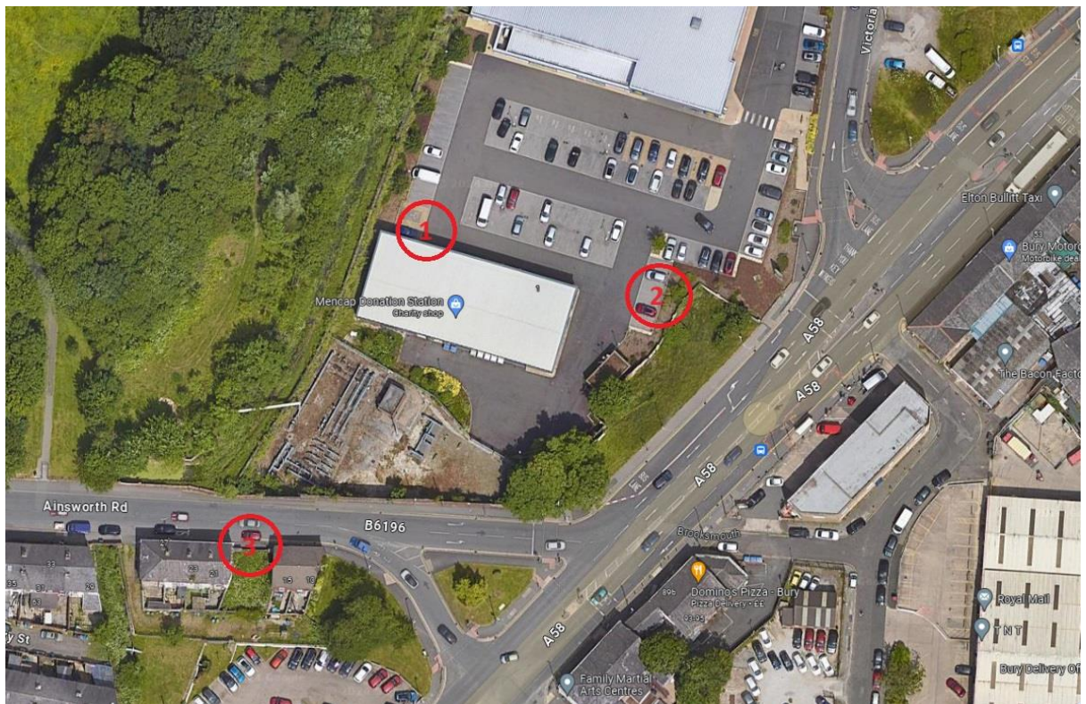
Figure 2 – Noise measurement positions around the Victoria Retail Park site.
