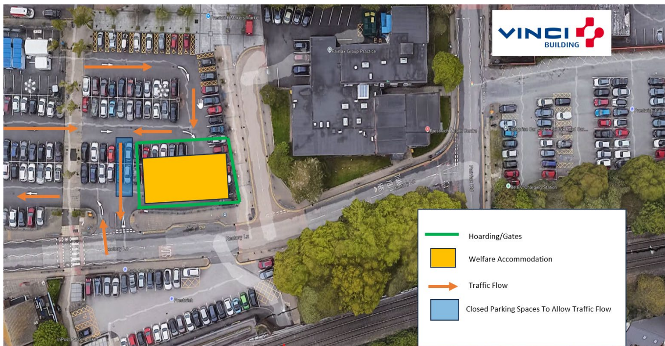
Figure 2.2.3- Site Compound Logistics Plan.
