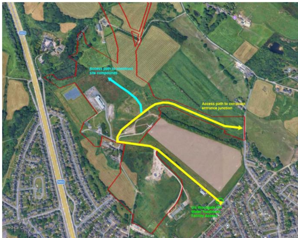
Image 5-1 Site Temporary Haul Road Design
