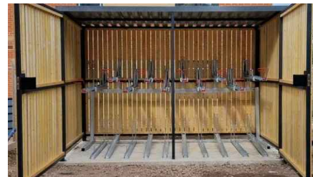
TIMBER TWO TIER BIKE SHELTER FOR MIN 6NO CYCLES. WOODEN CLADDING WITH A POWDER COATED GALVANISED STEEL FRAME, WITH ROOF OVER AND SECURE DOUBLE GATES. LOCKING HOPP PROVIDED FOR VERTICAL BIKE STORAGE, WITH RACKS BEING STAGGERED
