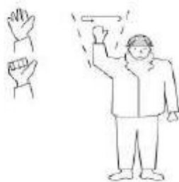
HOIST Clench and unclench fingers to 'inch' load
