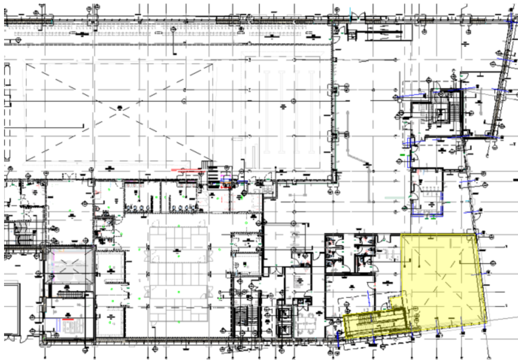
Basement 2 Titan bond radon membrane installation to basement floor and walls – Area of Installation/ Inspection for given date highlighted Yellow
