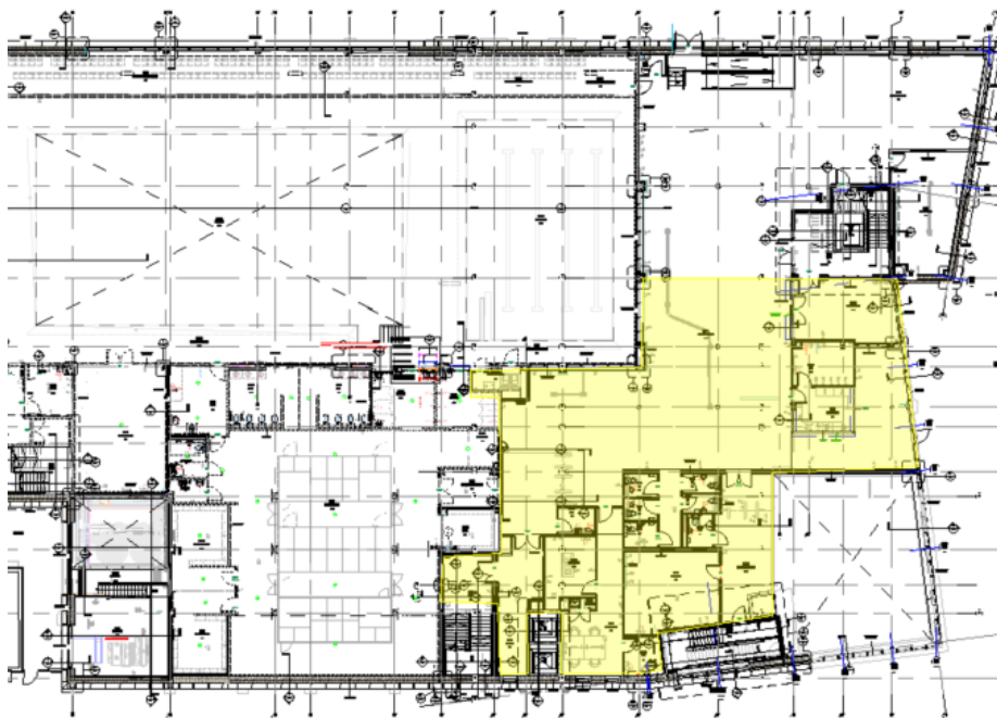
Phase 3 & 4 Floor slab area gas membrane install – Area of Installation/ Inspection for given date highlighted Yellow
