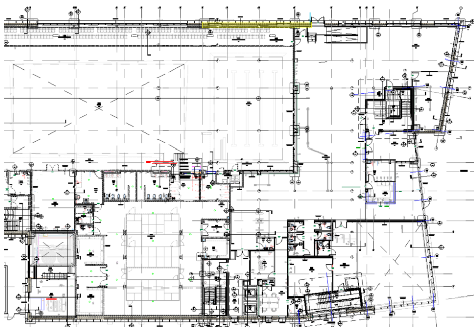
Ground floor northern external substructure around main pool (Liquid Gas Barrier) – Area of Installation/ Inspection for given date highlighted Yellow
