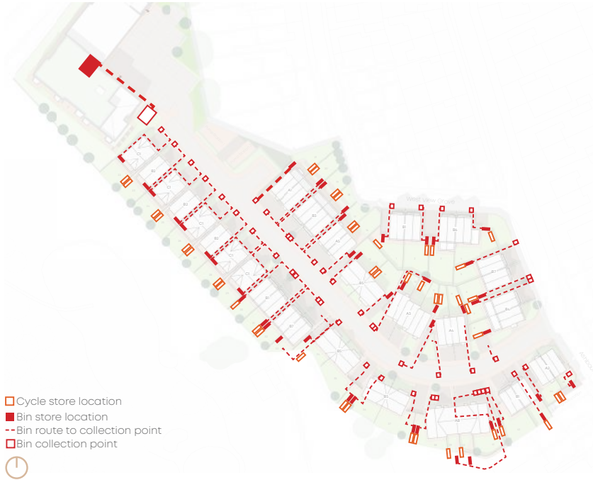
Fig.57 Cycle/bin store overlay [ PJA]
