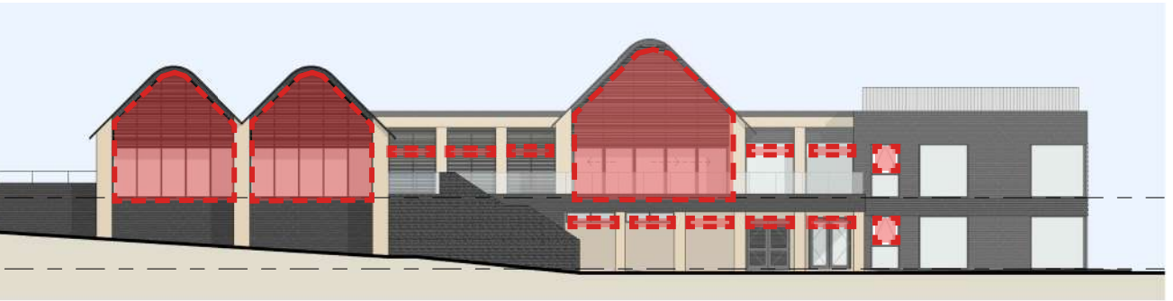
Fig.91 Areas explored for natural ventilation [PJA]
