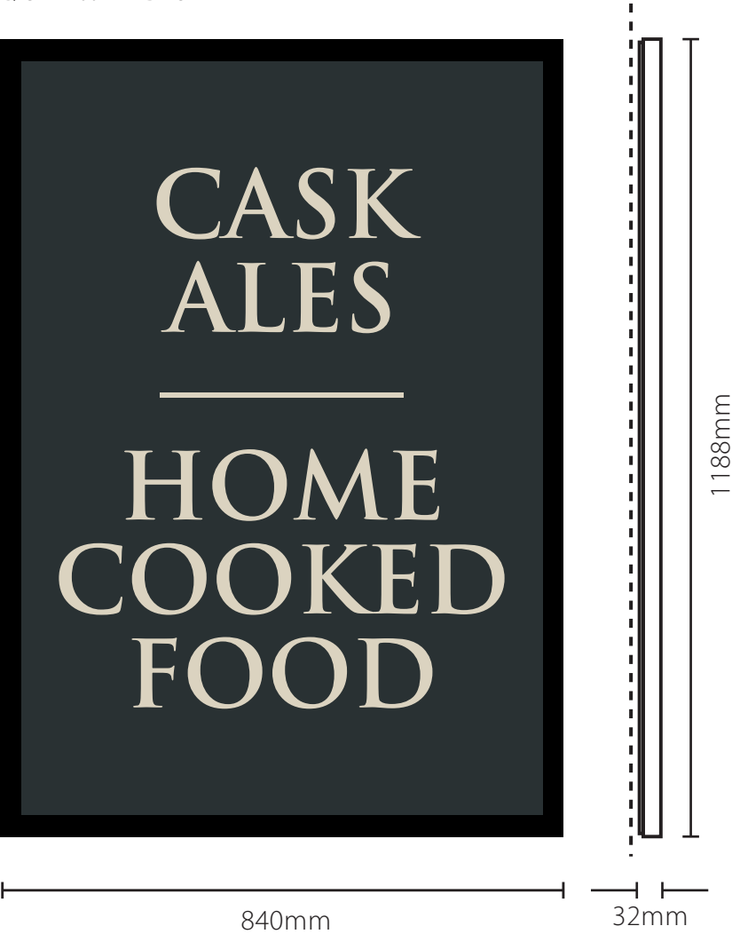
Scale : 1:10 @ A3 Item C. 1no. Sprayed Aluminium A0 poster case with applied vinyl. G/CI - 1200mm D - 32mm
