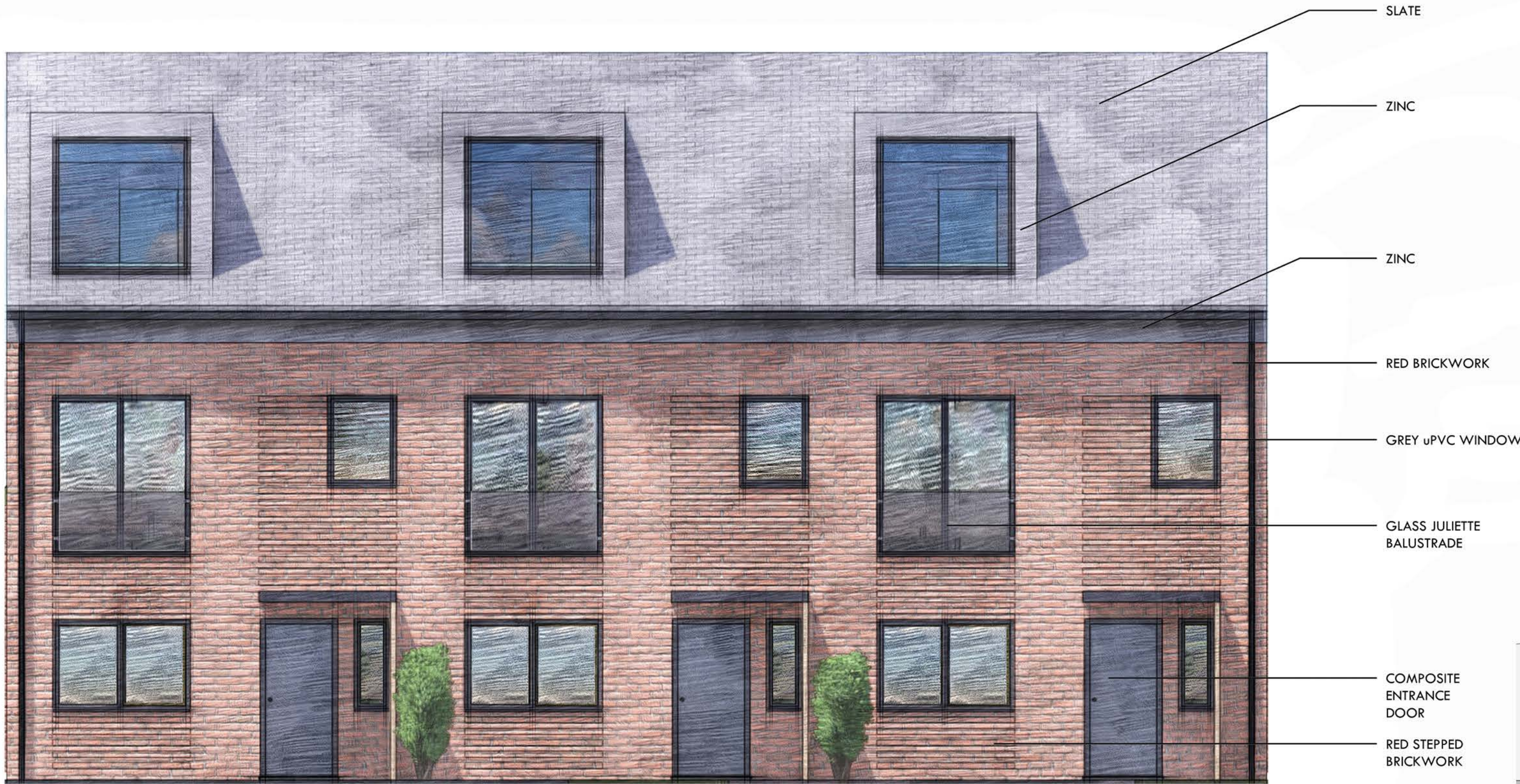
Front Elevation (North)
