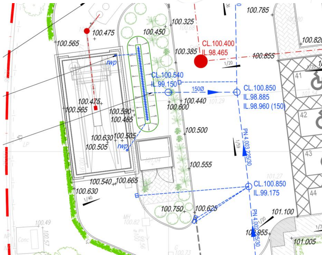
Figure 8 Extract from proposed drainage layout
