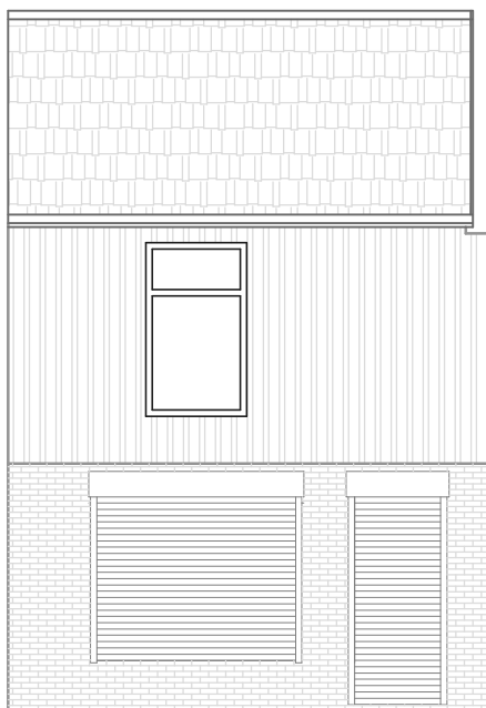
EXISTING FRONT ELEVATION WHILE SHUTTERS DOWN
