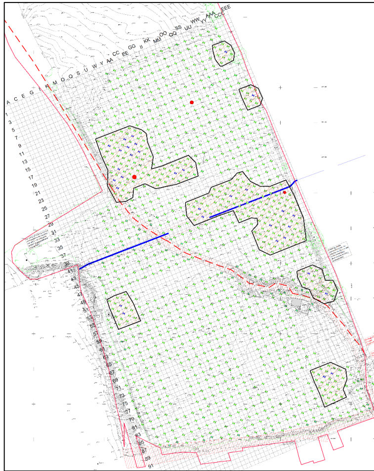
Extract of the completed drill and grout grid with areas requiring secondary holes outlined and highlighted in orange.
