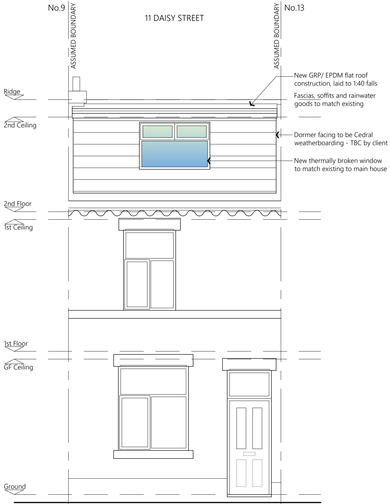
PROPOSED FRONT ELEVATION NO CHANGES TO REAR ELEVATION
