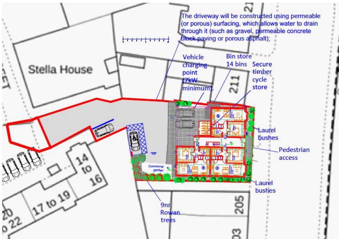
Fig 8 – Existing building line is respected
