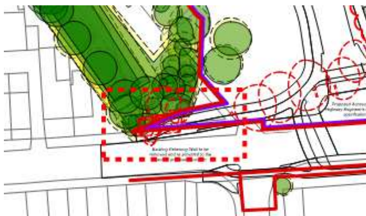
Figure 3.2 – New Retaining Wall Location Plan
