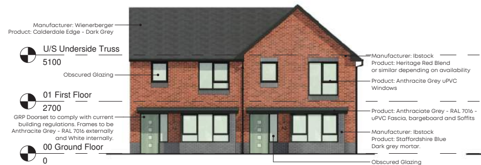
Typical House Front Elevation
