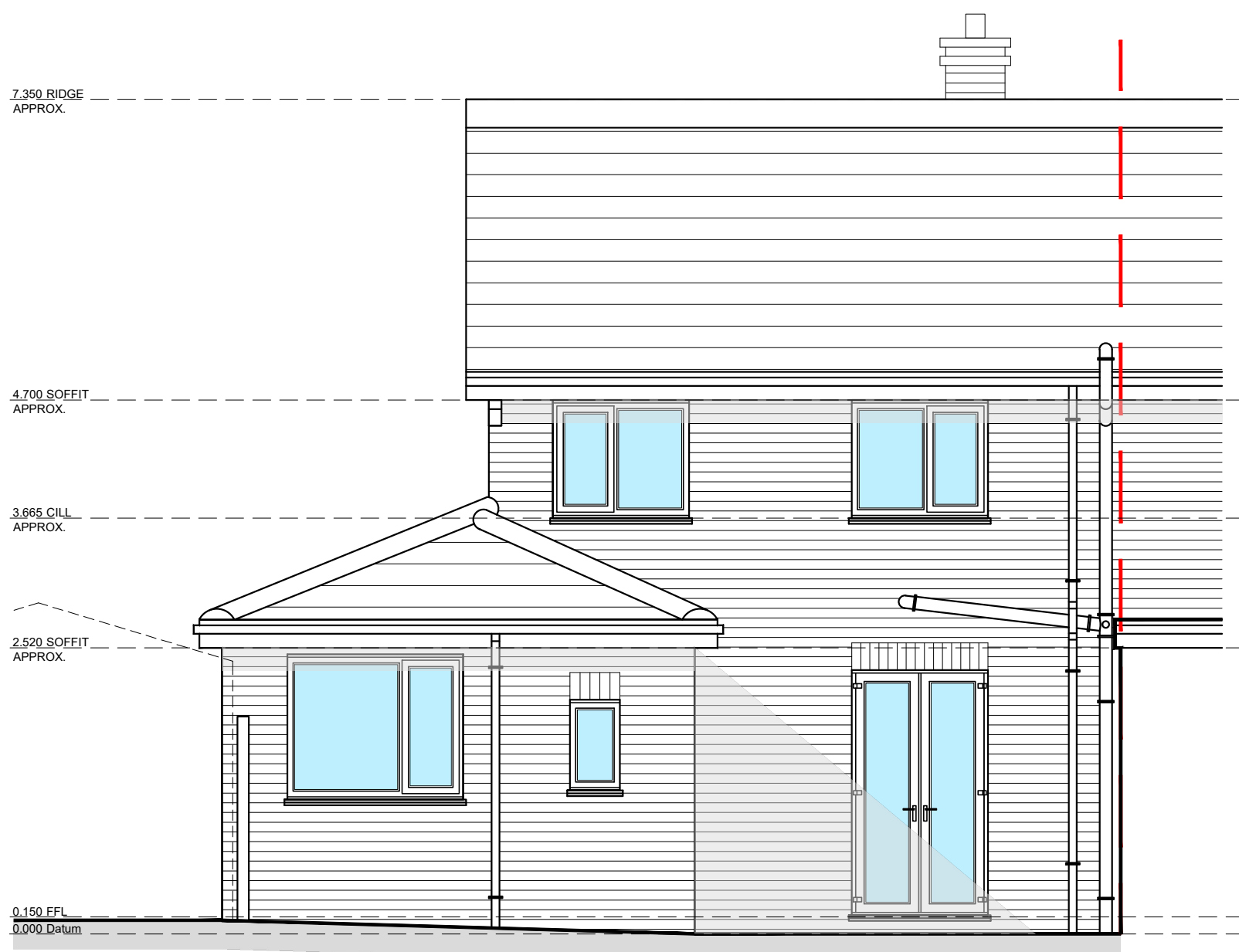
Existing Rear Elevation (C) 1:50
