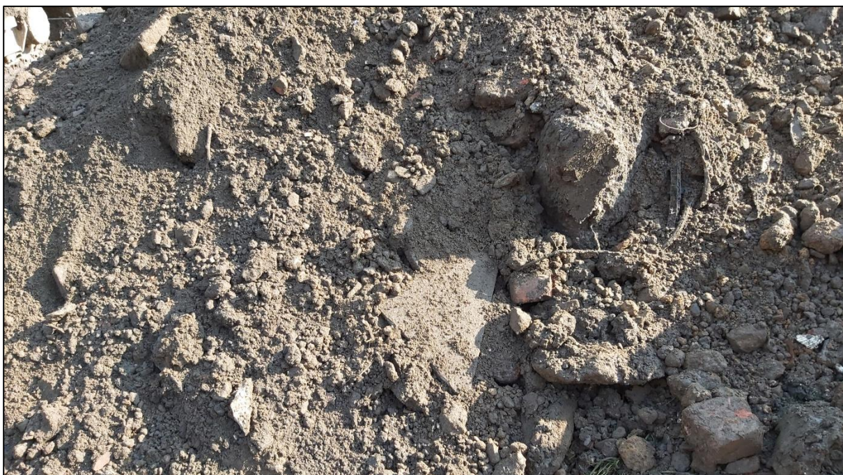
Photograph 7 – TP3 Spoil of Made Ground
