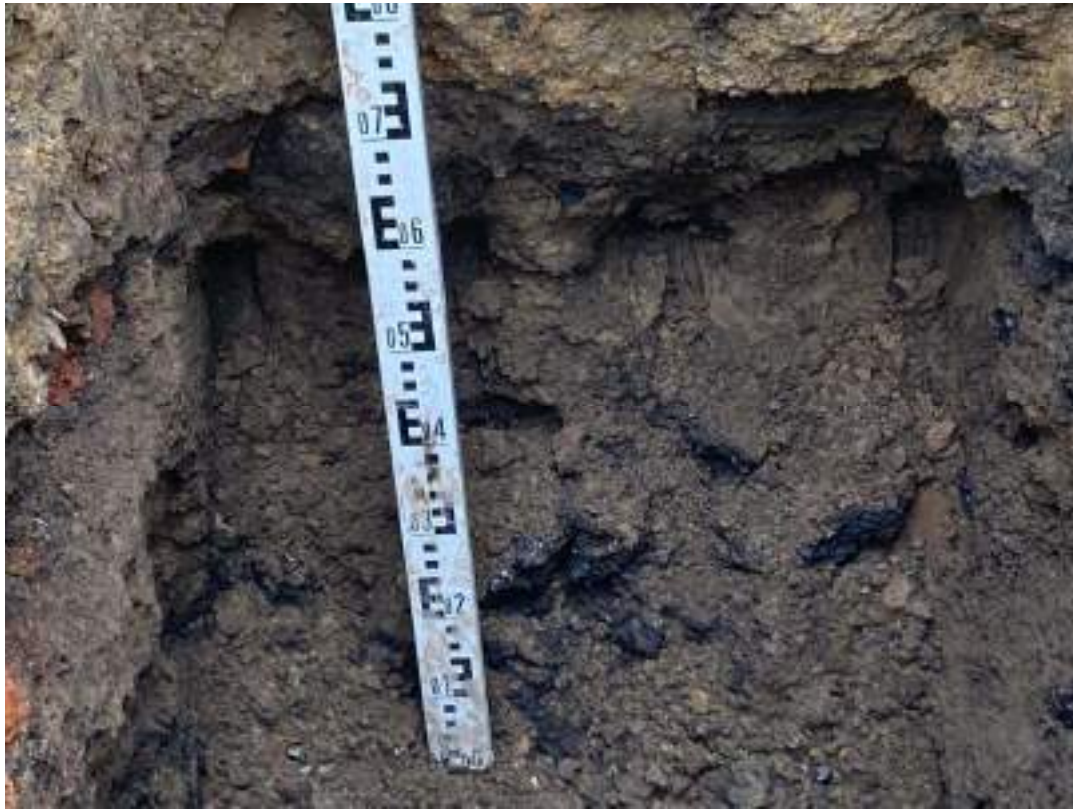
Plate 17 – TP4 natural ground with coal cobbles
