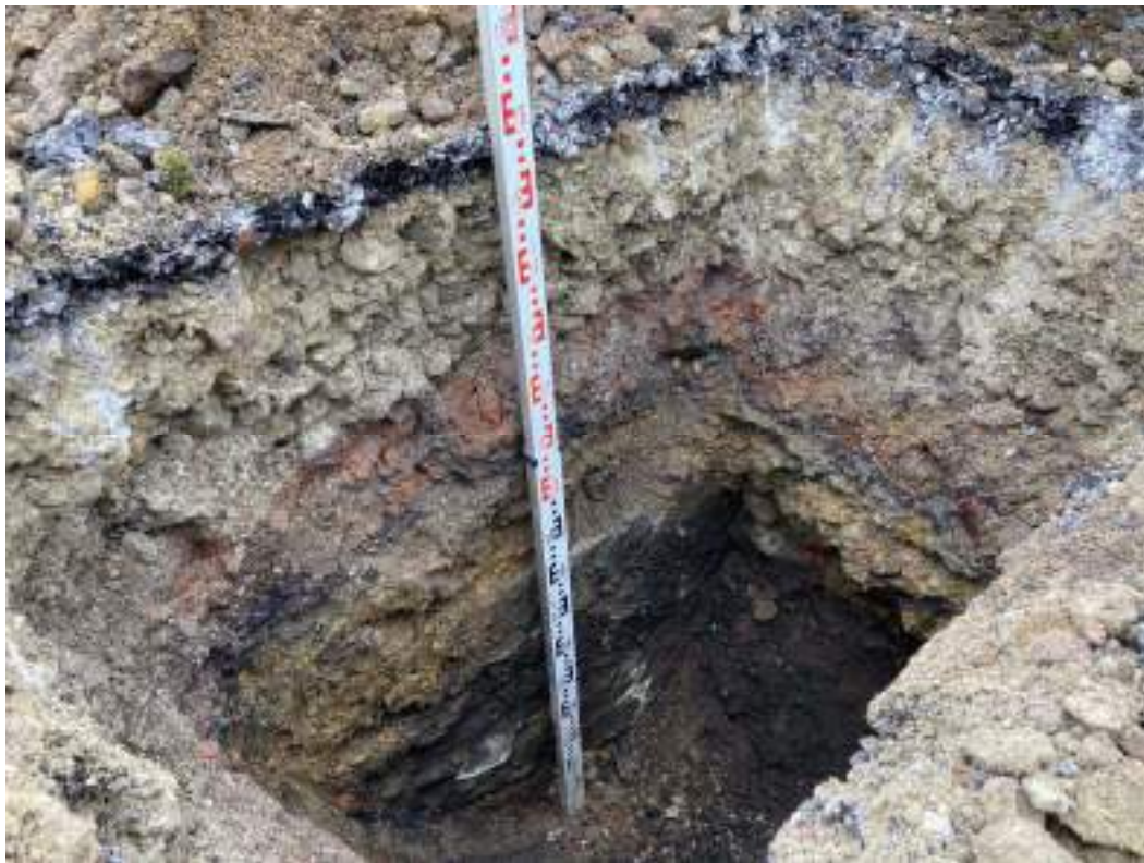
Plate 16 – TP4 west face (left) and north face (right) gl to 1.6mbgl
