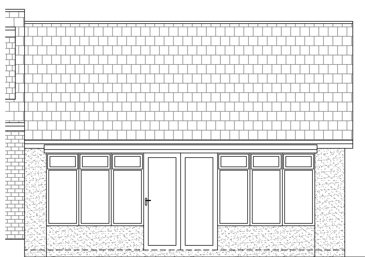
Existing Rear Elevation (1:50)
