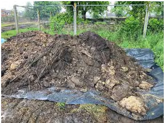
PLATE 5 STOCKPILED ARISINGS FROM WS104 – HOTSPOT 1
