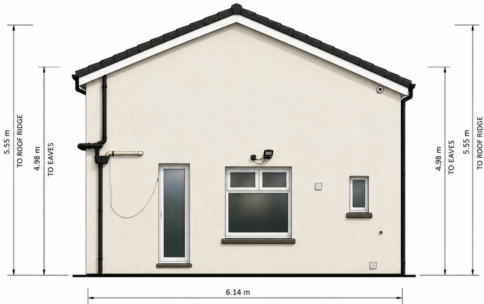
EXISTING SIDE ELEVATION 1:100
