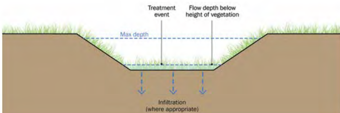
Figure 12 – Typical conveyance/attenuation swale (CIRIA, 2015)
