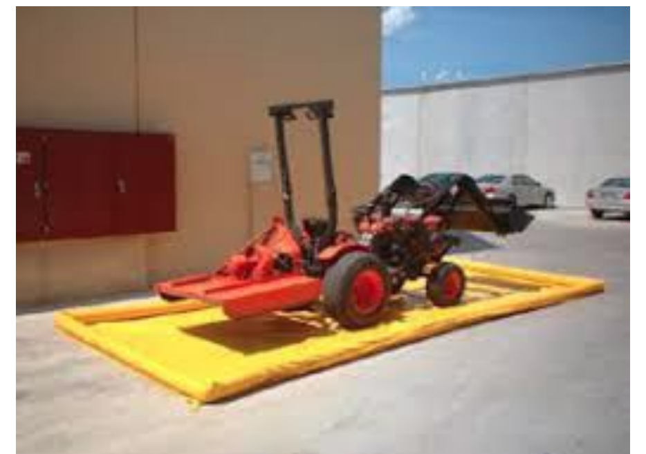
Examples of wheel wash enclosures
