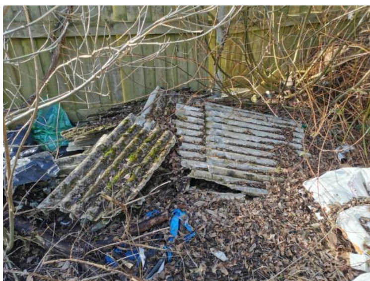
Plate 14 - Dumped asbestos along the western boundary
