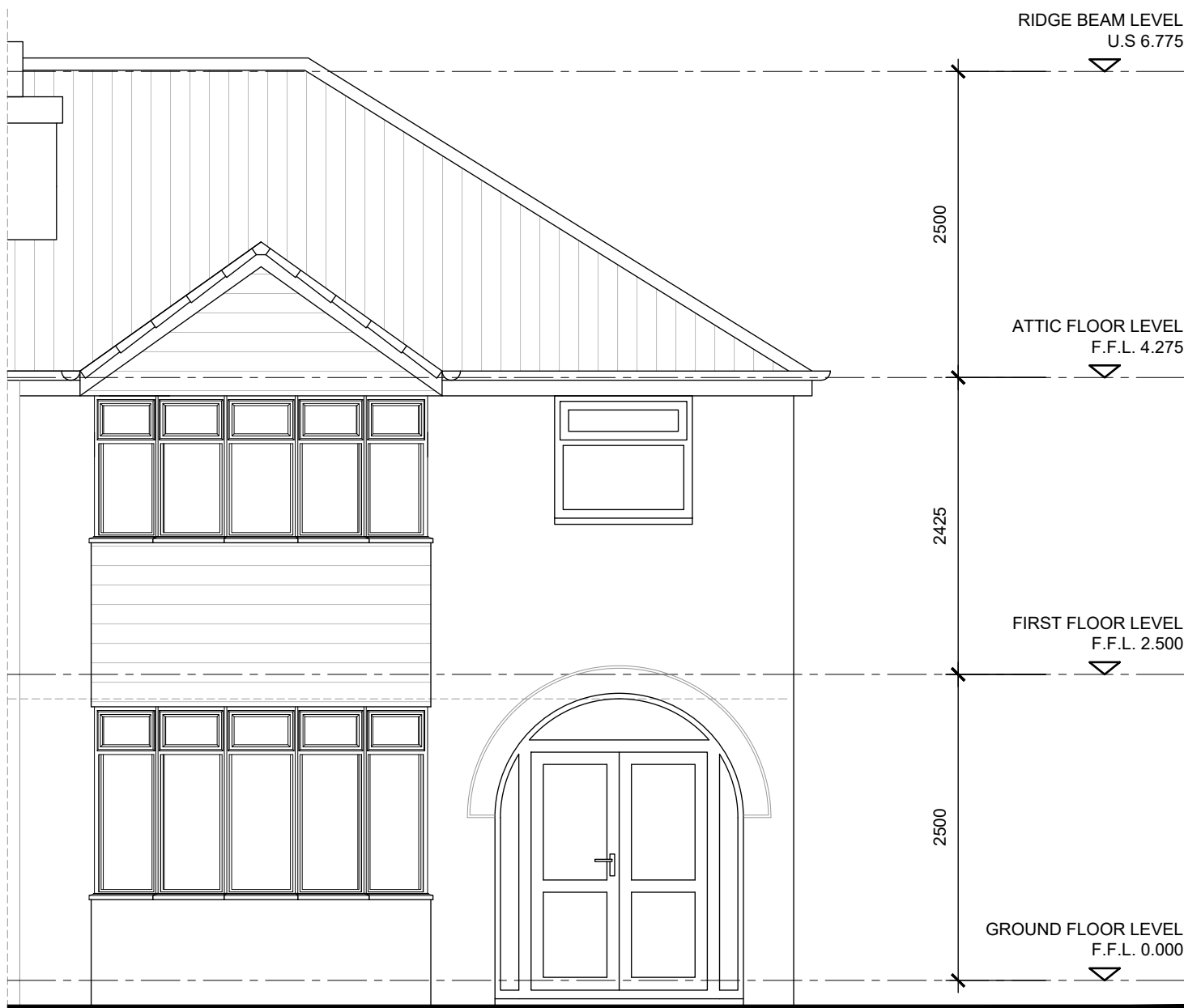
EXISTING FRONT ELEVATION
