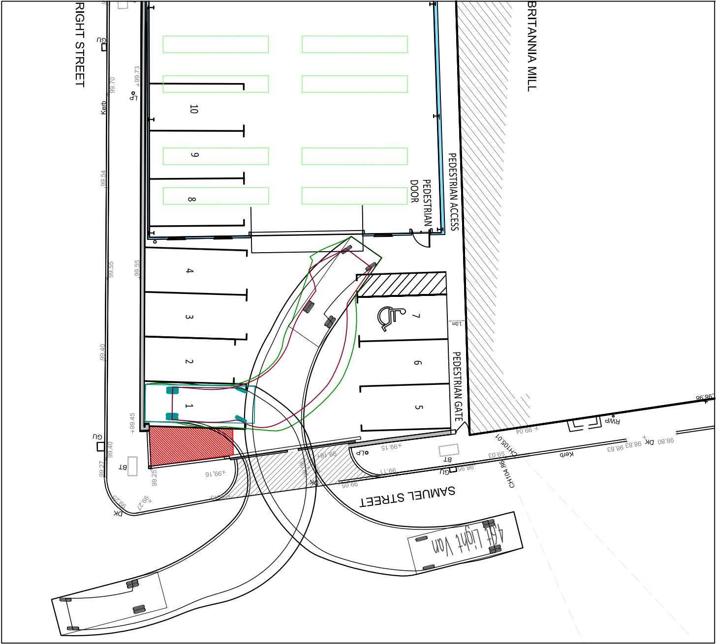
SWEPT PATH INDICATING TRANSIT VAN DELIVERY MANOUEVERS
