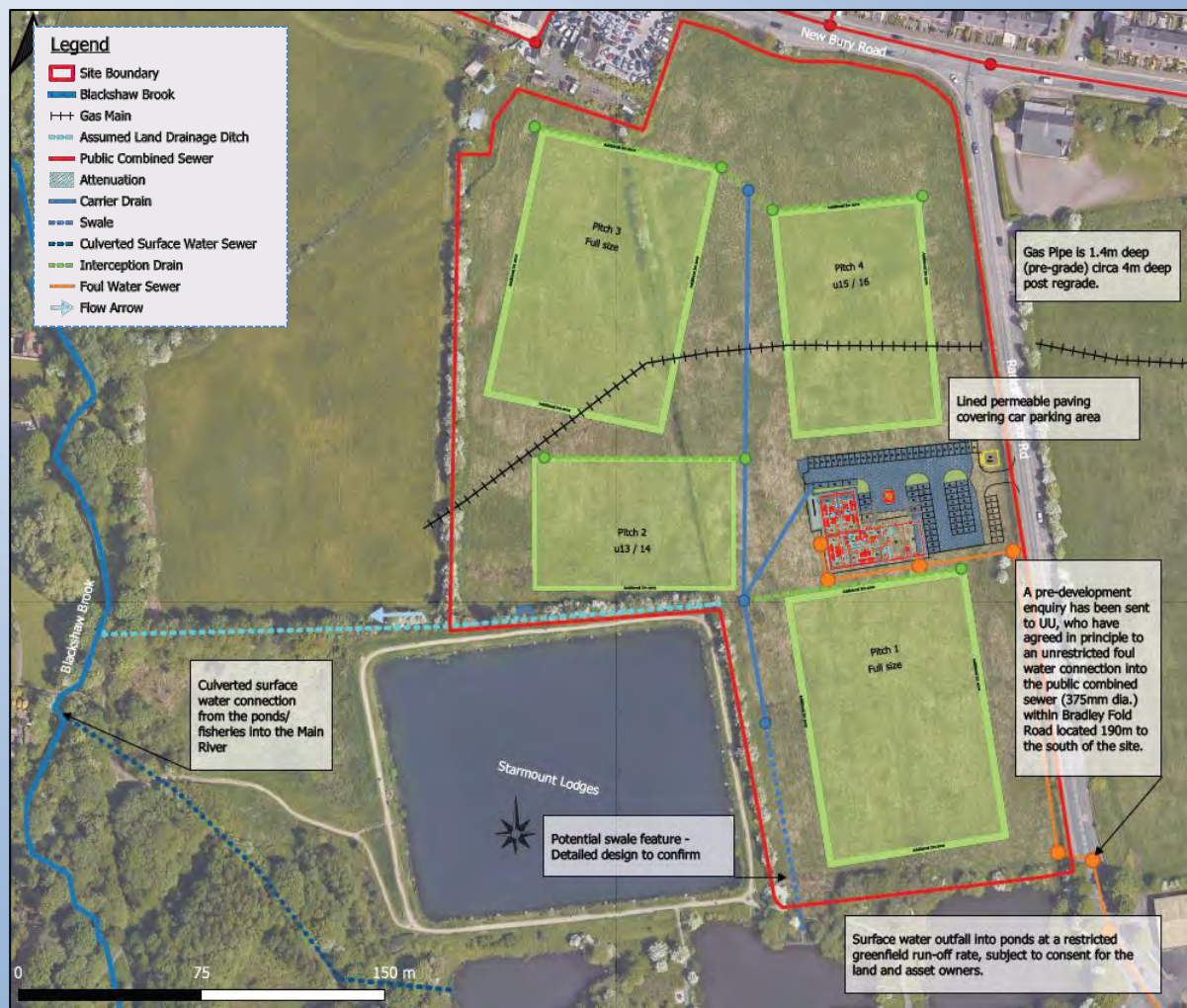
Figure 3: Preliminary Proposed Drainage Plan (Betts Hydro, 2021)
