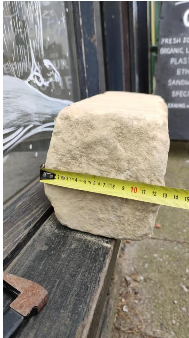
Proposed stone thickness: approx.. 130mm
