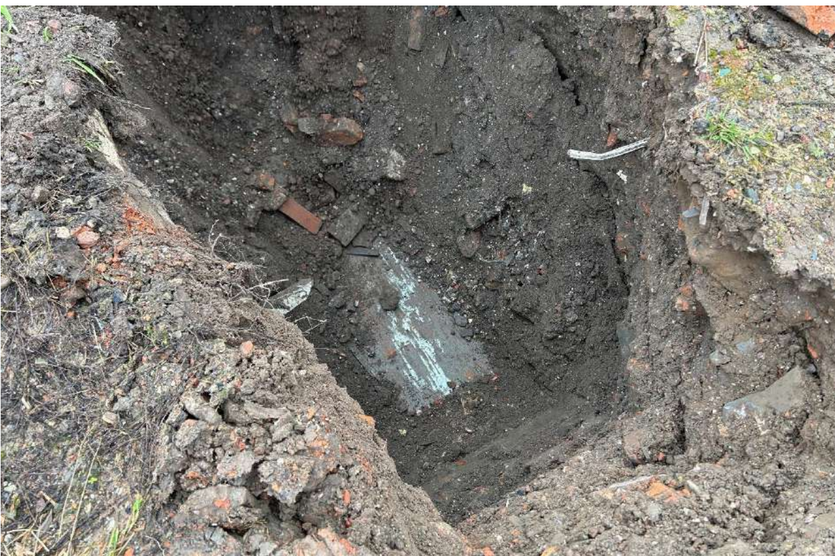
Photograph 22 – TP05 showing the depth of the basement at 1.90m bgl.
