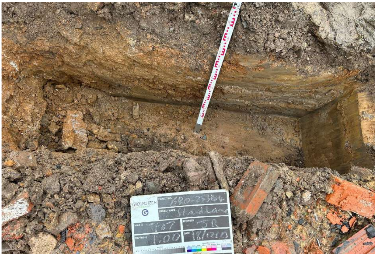
Photograph 25 – TP07 indicates the basement does not extend to the edge of the site on the north eastern boundary.
