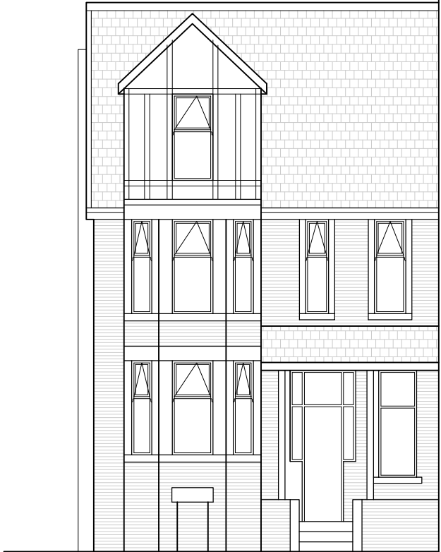
EXISTING FRONT ELEVATION 1 : 125 @ A3
