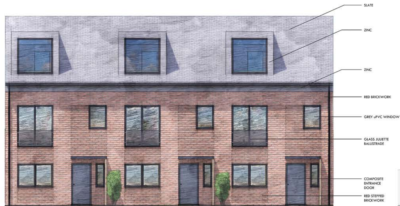
Front Elevation (North) 1 : 50
