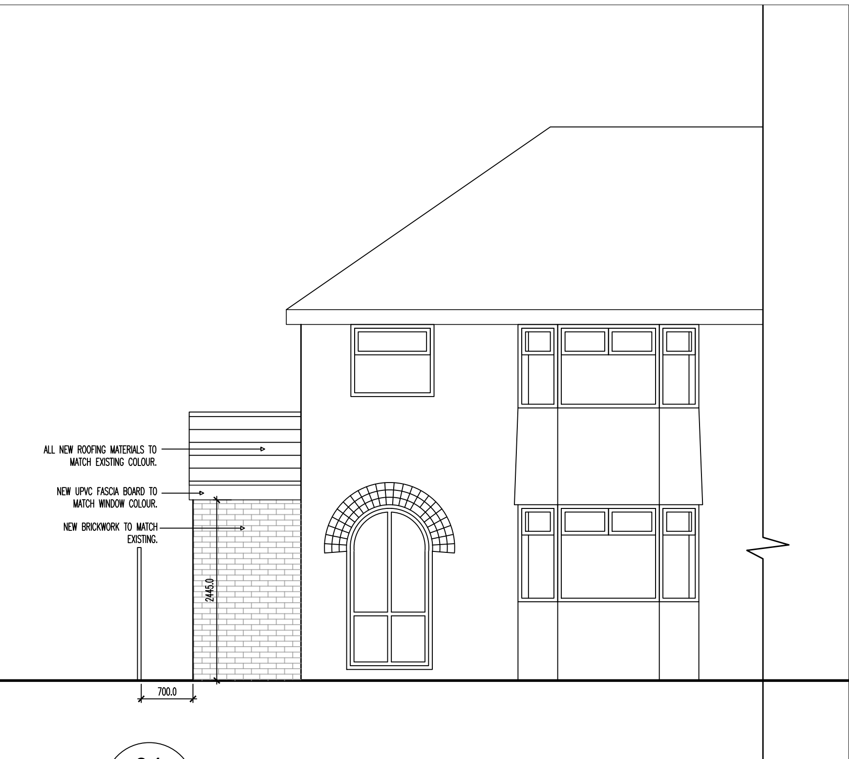
04 Proposed Front Elevation Scale 1:50
