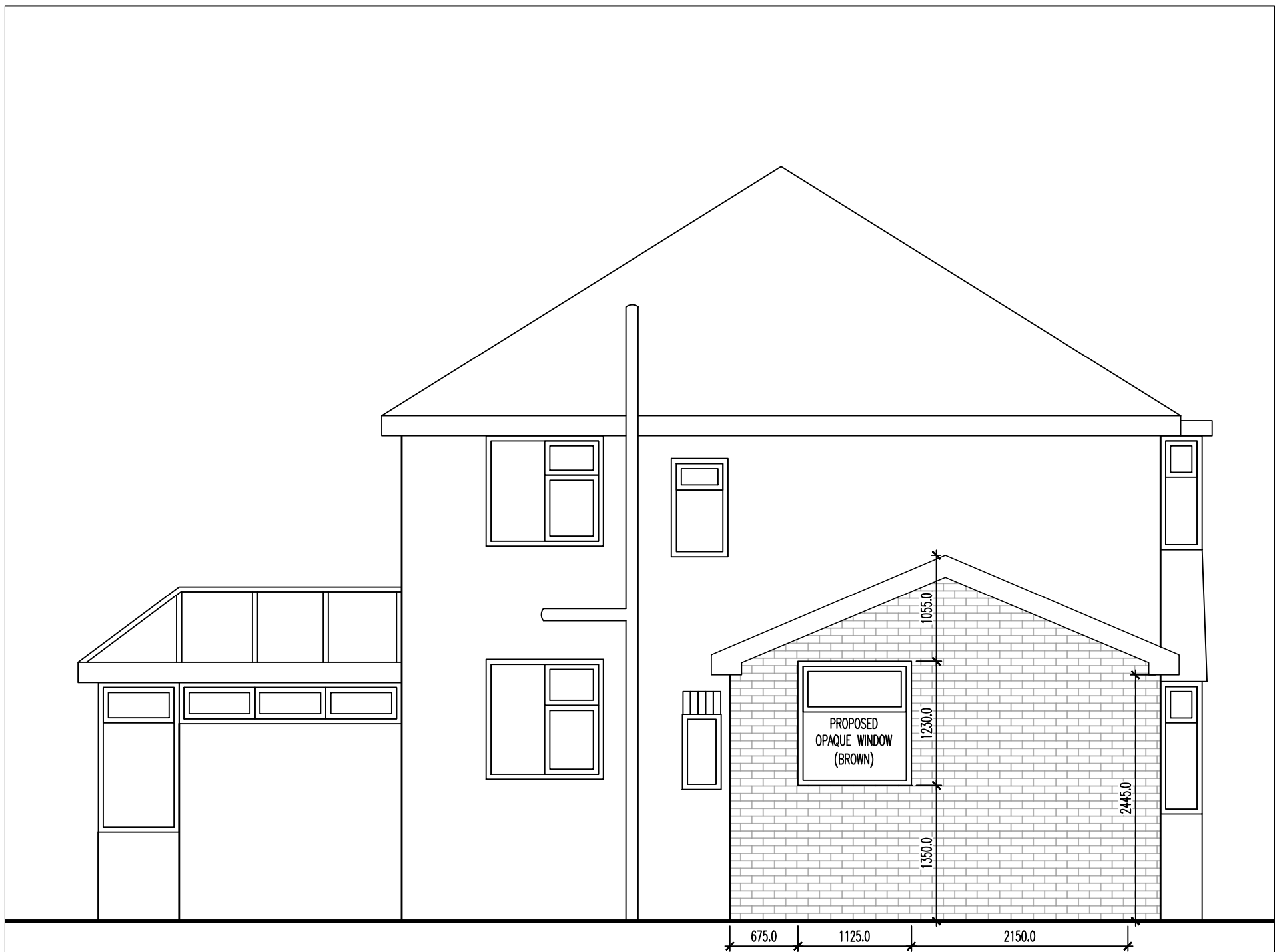
03 Proposed Side Elevation Scale 1:50
