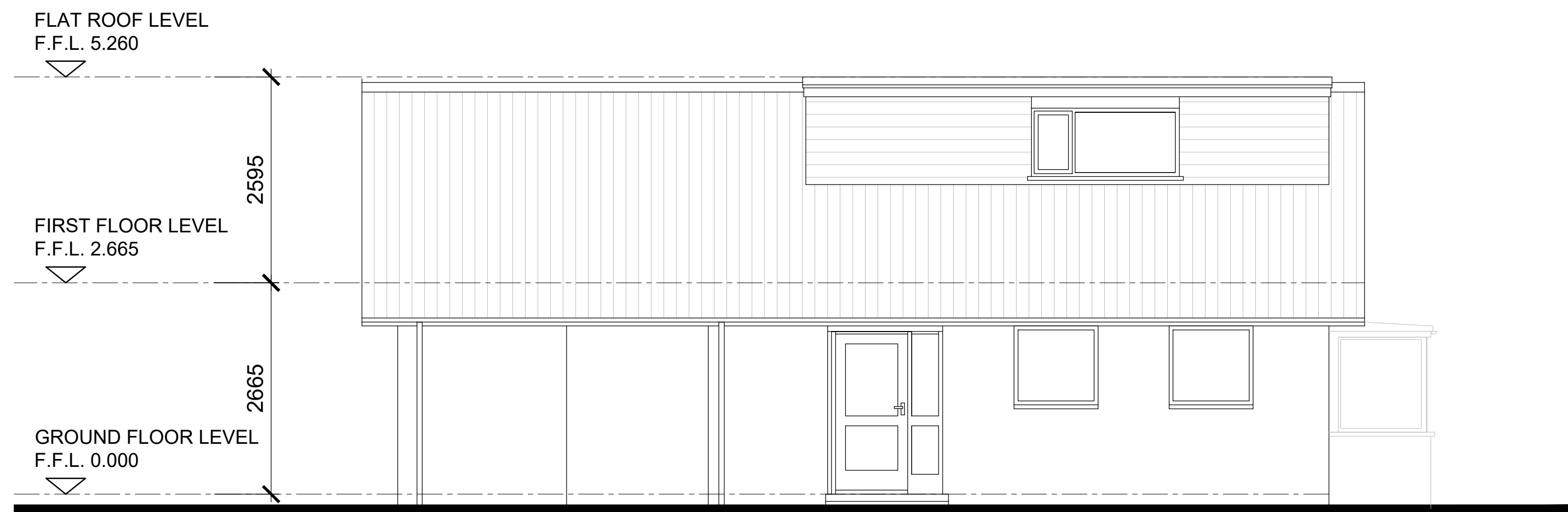
EXISTING SIDE ELEVATION
