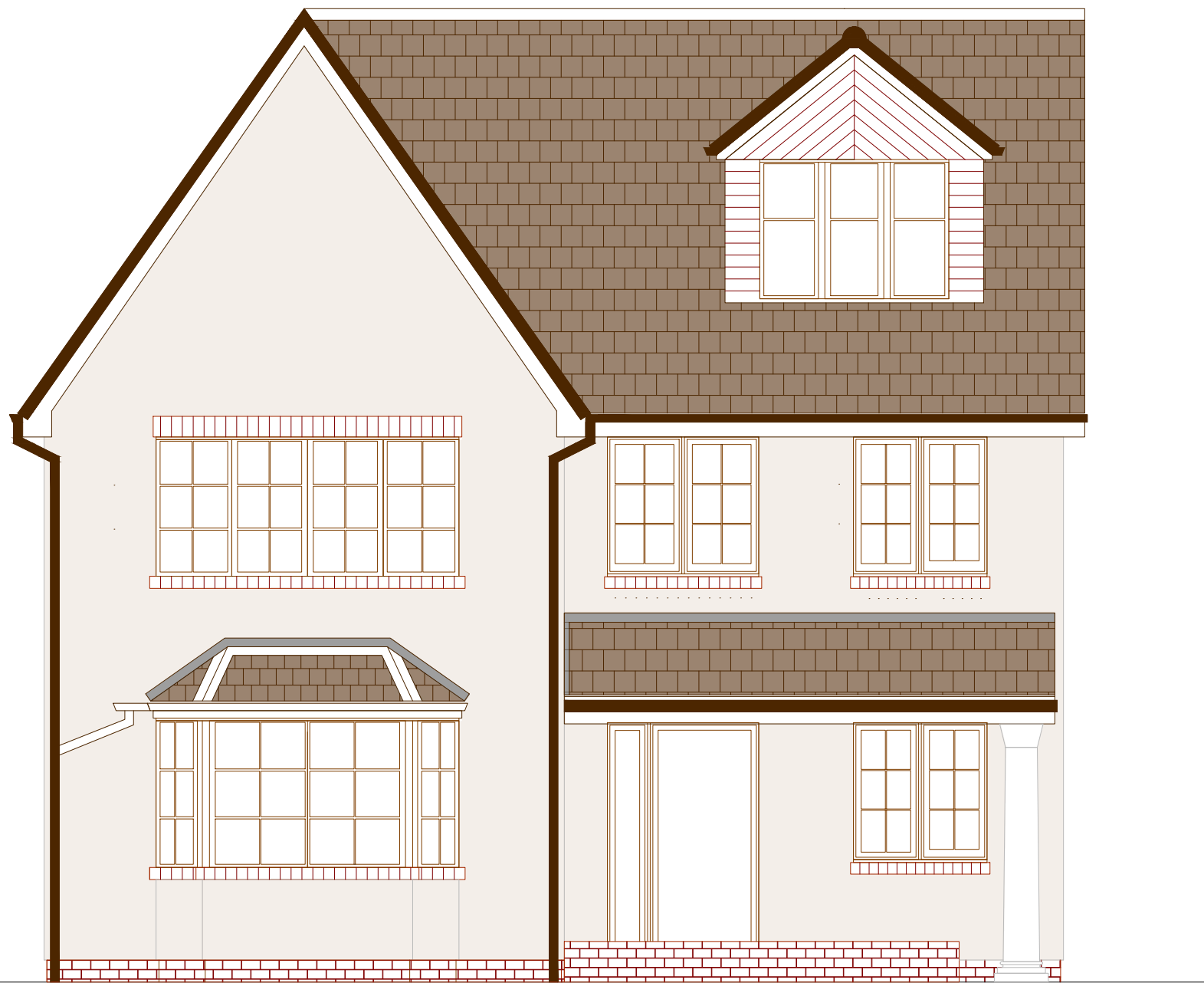
EXISTING FRONT ELEVATION
