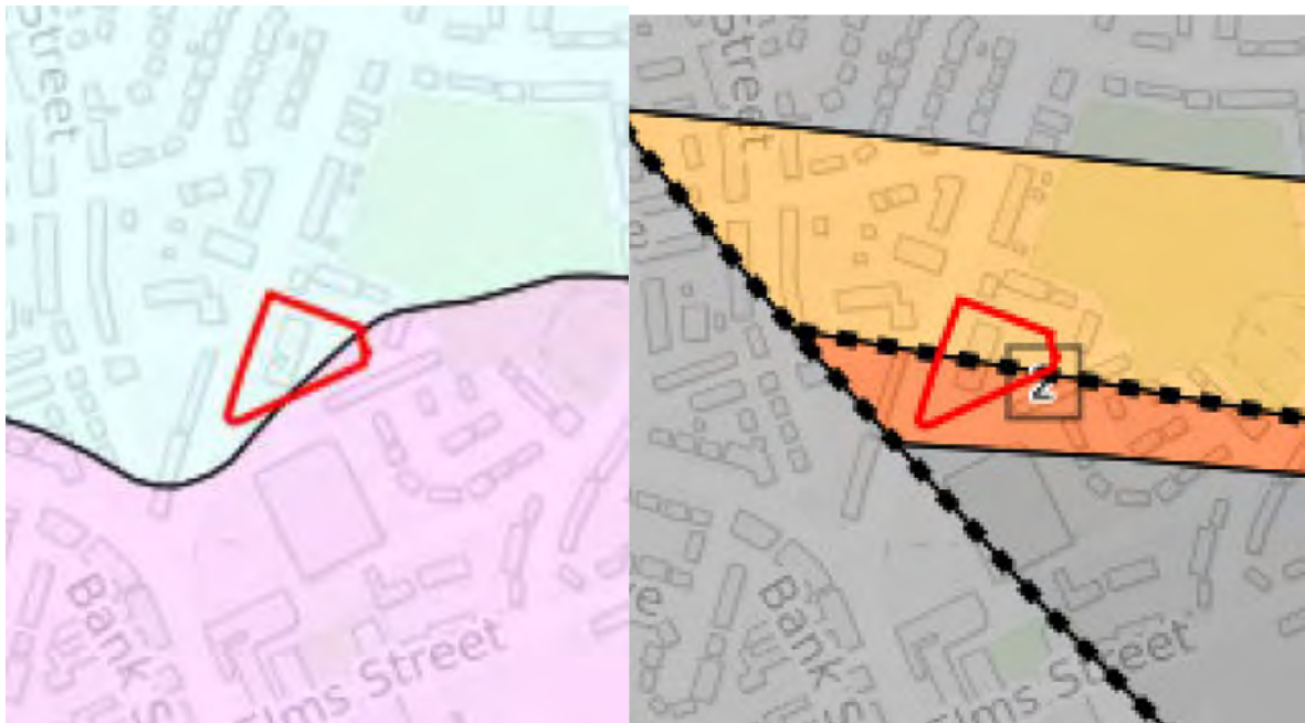
Figure 8: Extracts of the BGS 1:50,000 Drift (left) and Solid (right) Geological Maps. Light blue = Glacial Till, Pink = Glaciofluvial Deposits. Light Orange = Collyhurst Sandstone Formation, Dark Orange = Manchester Marls Formation
