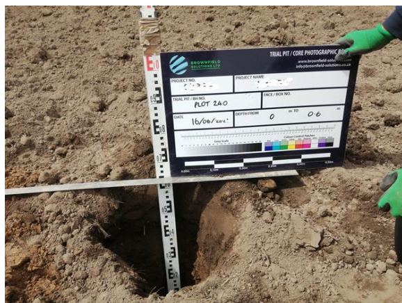
Evidence of Hard Dig Layer
