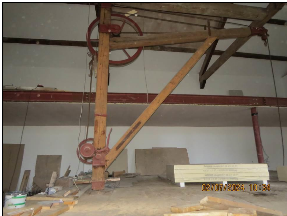
025 Hoist general arrangement, chainage 10 – 13 metres
