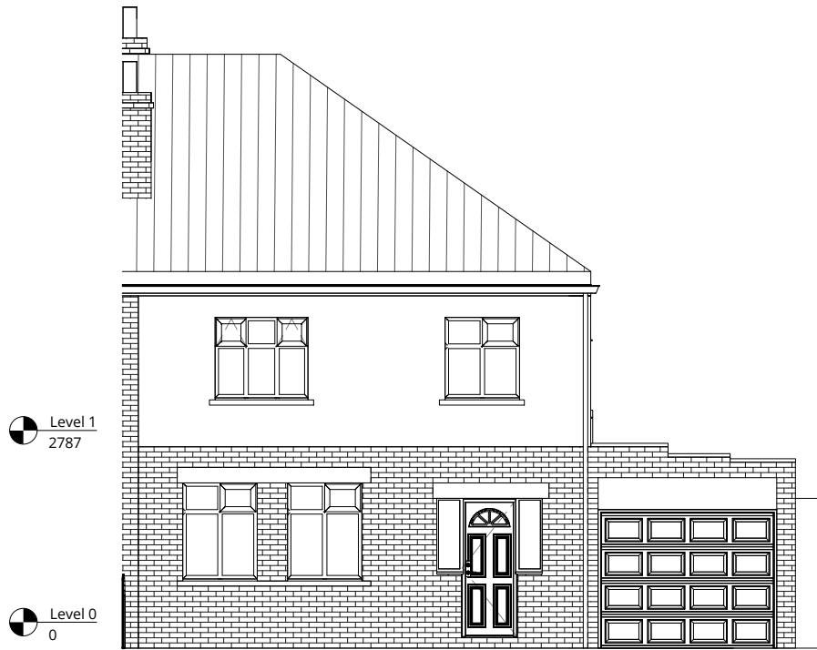
3 Existing Front Elevation 1 : 100
