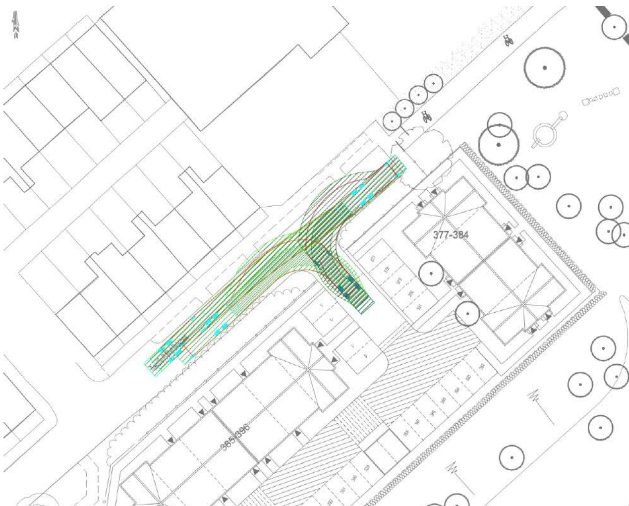
Figure 2.3 – Brook Street Swept Path Analysis
