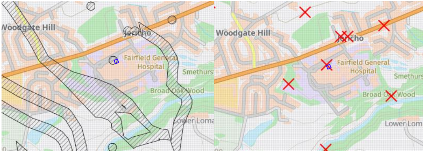
Figure 3 – Mining Remediation Authority Recorded Development High Risk Area (Left) Highlighted in Black Hatching. Mining Remediation Authority Recorded Mine Entries (right) Highlighted by Red X. Approximate Site Boundary in Red.
