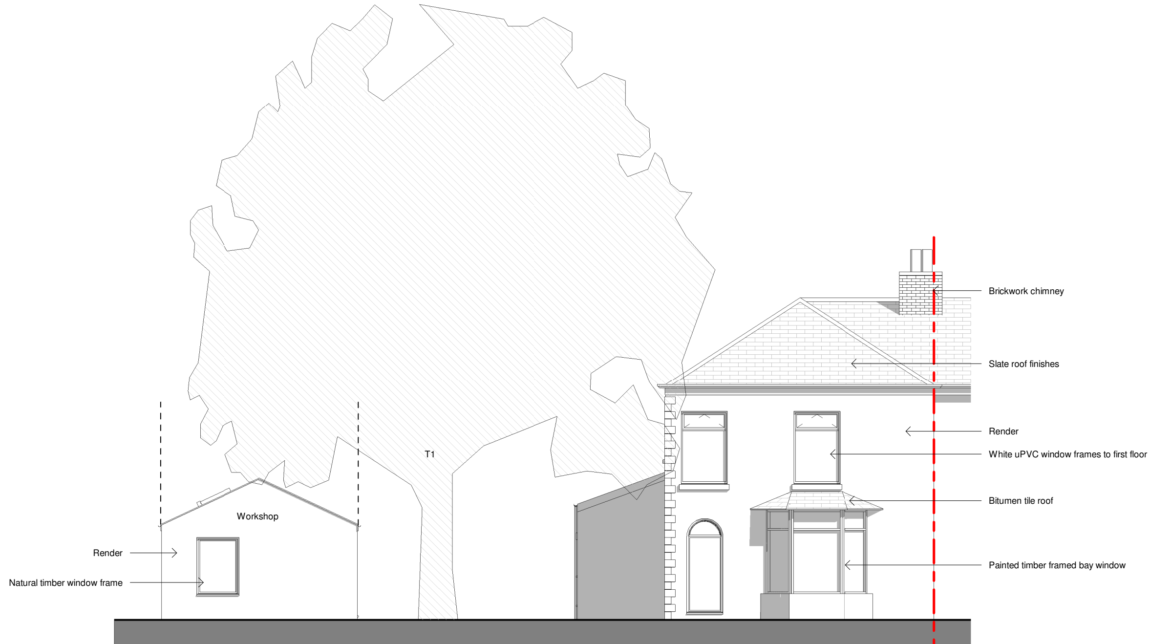
1 Existing South Elevation 1 : 100
