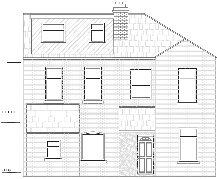
Existing Rear Elevation
