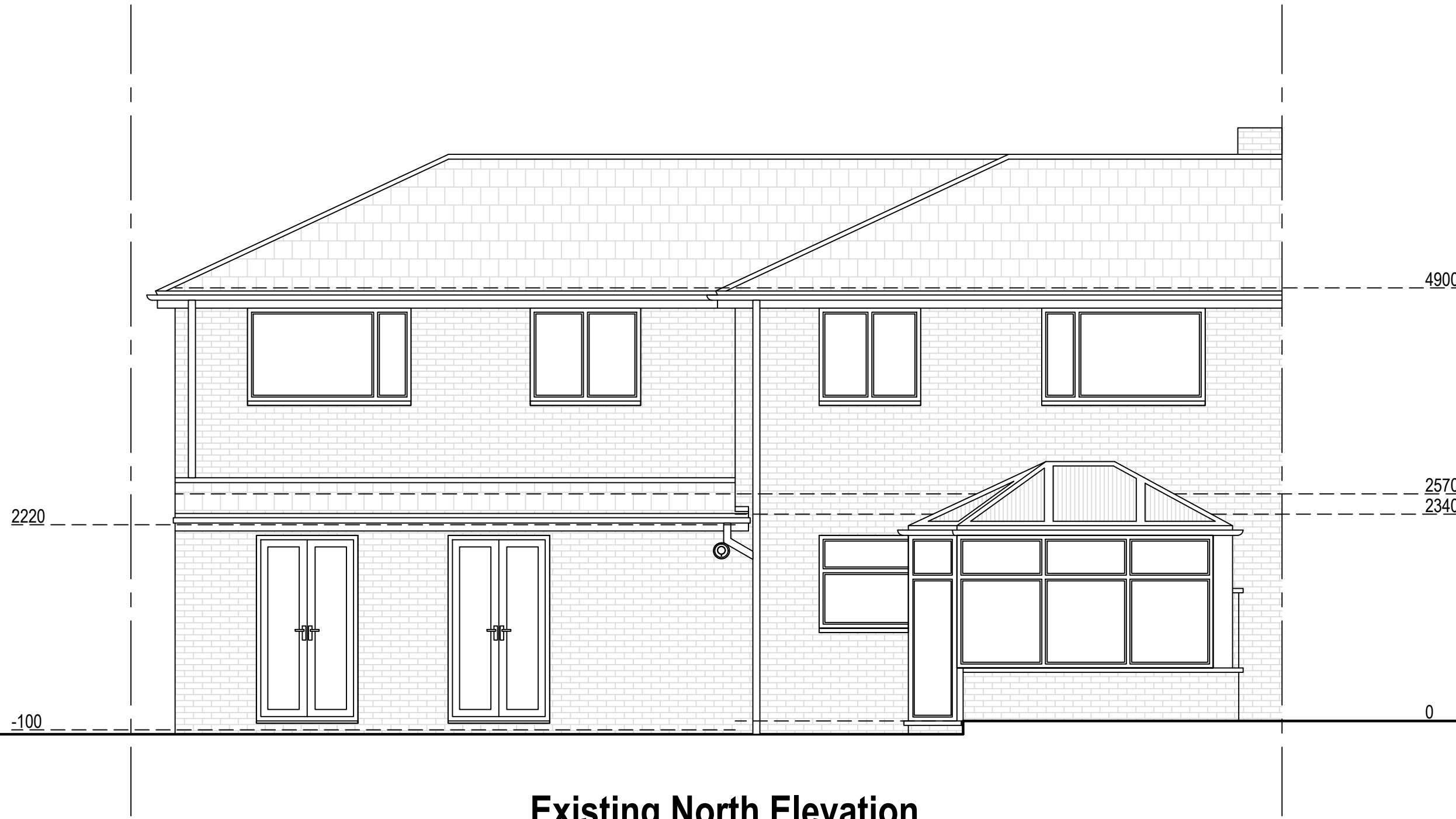
Existing North Elevation
