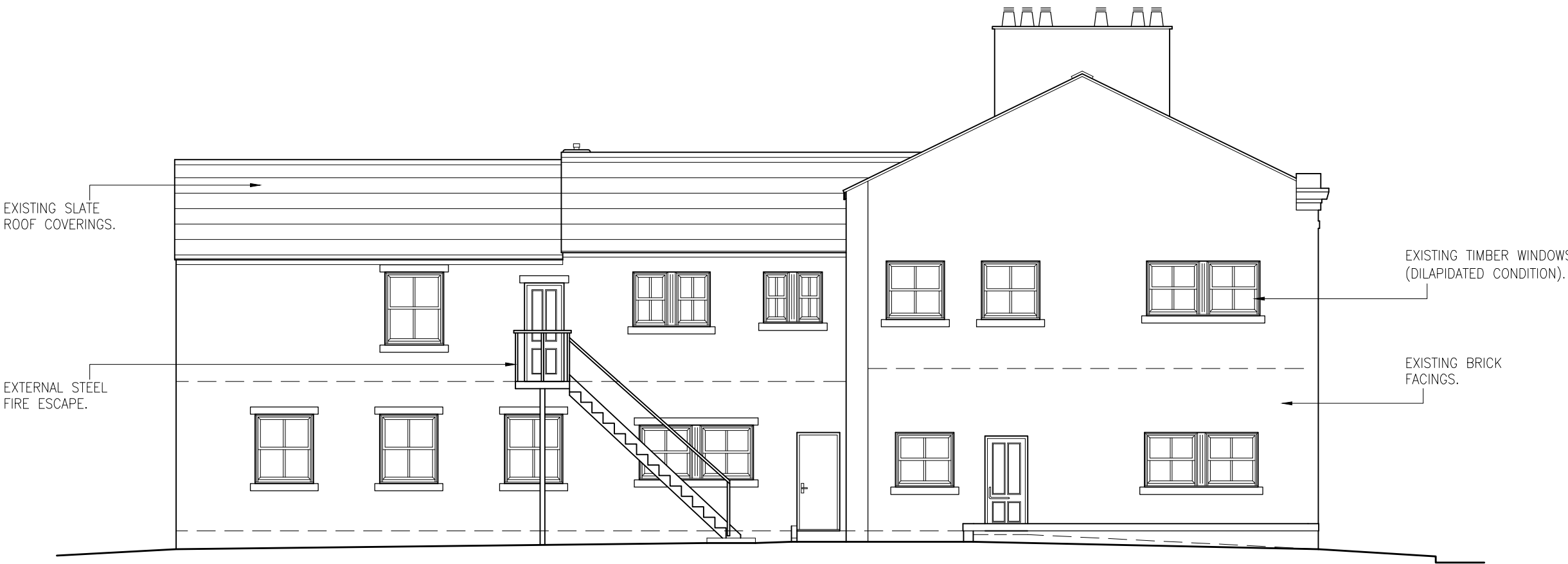
EXISTING SIDE/WEST ELEVATION (1:100)
