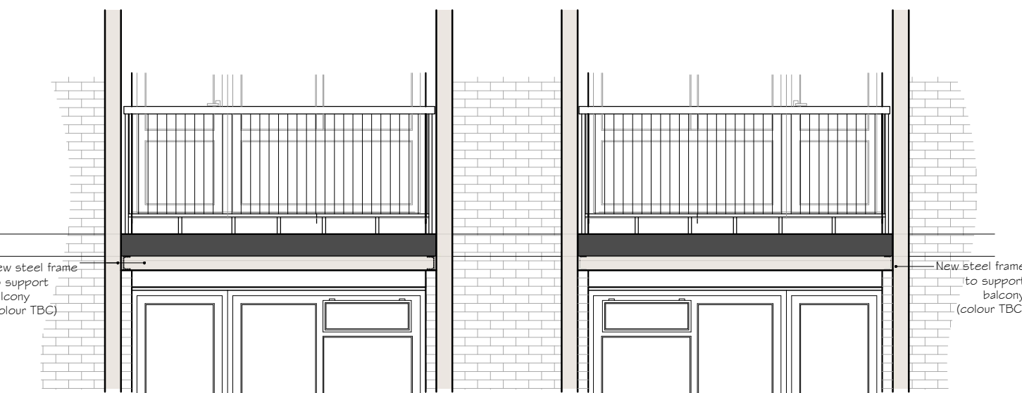
Elevation of Balcony B2 as Proposed
